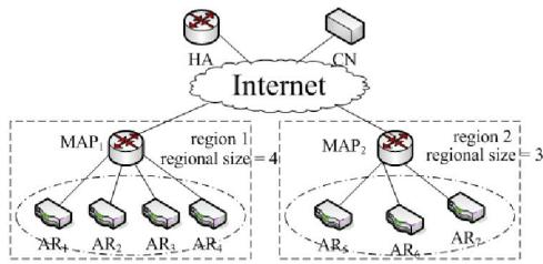
Fig. 1. Framework of HMIPv6.
