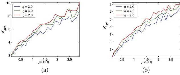
Fig. 9. Impact of wired/wireless delivery delay on the average value of  $K_{opt}$ .
