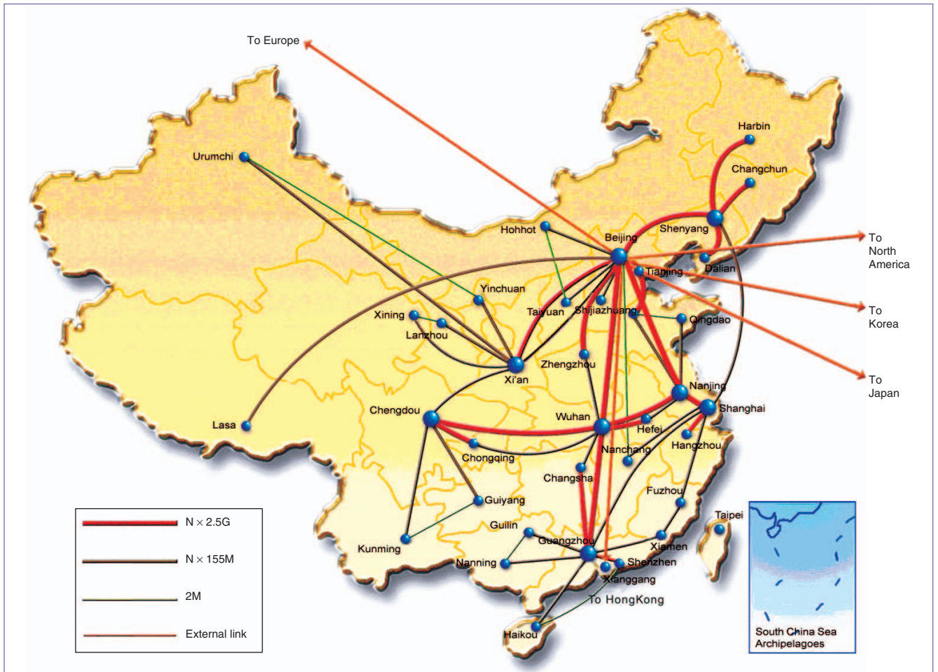
Figure 1. The China Education and Research Network. CERNET's topology includes roughly 40 points-of-presence that form a backbone with bandwidths ranging from 10 Gbits down to 2.5 Gbits at the regional level, supporting many national network applications, including distance learning, digital libraries, and grid computing.
